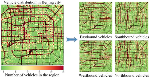
Fig. 2. The vehicle data is distinguished according to the driving direction to form a tensor  $F_t$ .
