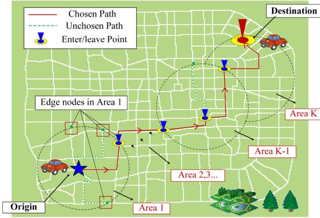
Fig. 5. The entire process of the gridded path planning algorithm.
