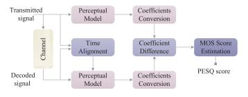
Fig. 12. Basic diagram of PESQ.
