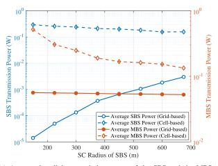
(a) Average downlink transmission power of the SBS and the MBS versus SC radius.
