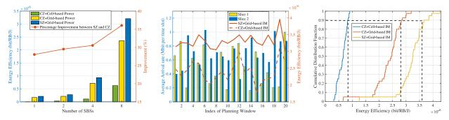
(a) Average network energy efficiency versus the (b) Temporal variations in data traffic load and (c) The cumulative distribution function of netnumber of SBSs. network energy efficiency. work energy efficiency.
