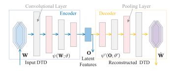
Fig. 5. The designed DNN architecture of the auto-encoder.
