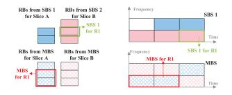
(a) Virtual slice separation in the plan- (b) RB allocation in the operation ning stage.
