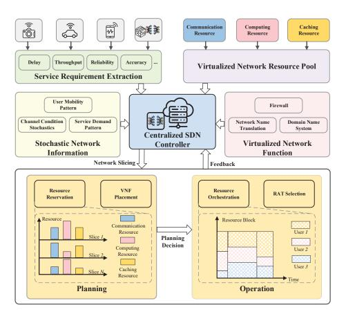
Fig. 2. An illustrative example for the network slicing lifecycle which includes preparation, planning, and operation phases.
