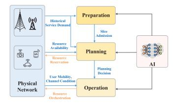
Fig. 3. The considered AI-based network slicing solution in which AI plays different roles in preparation, planning, and operation phases.
