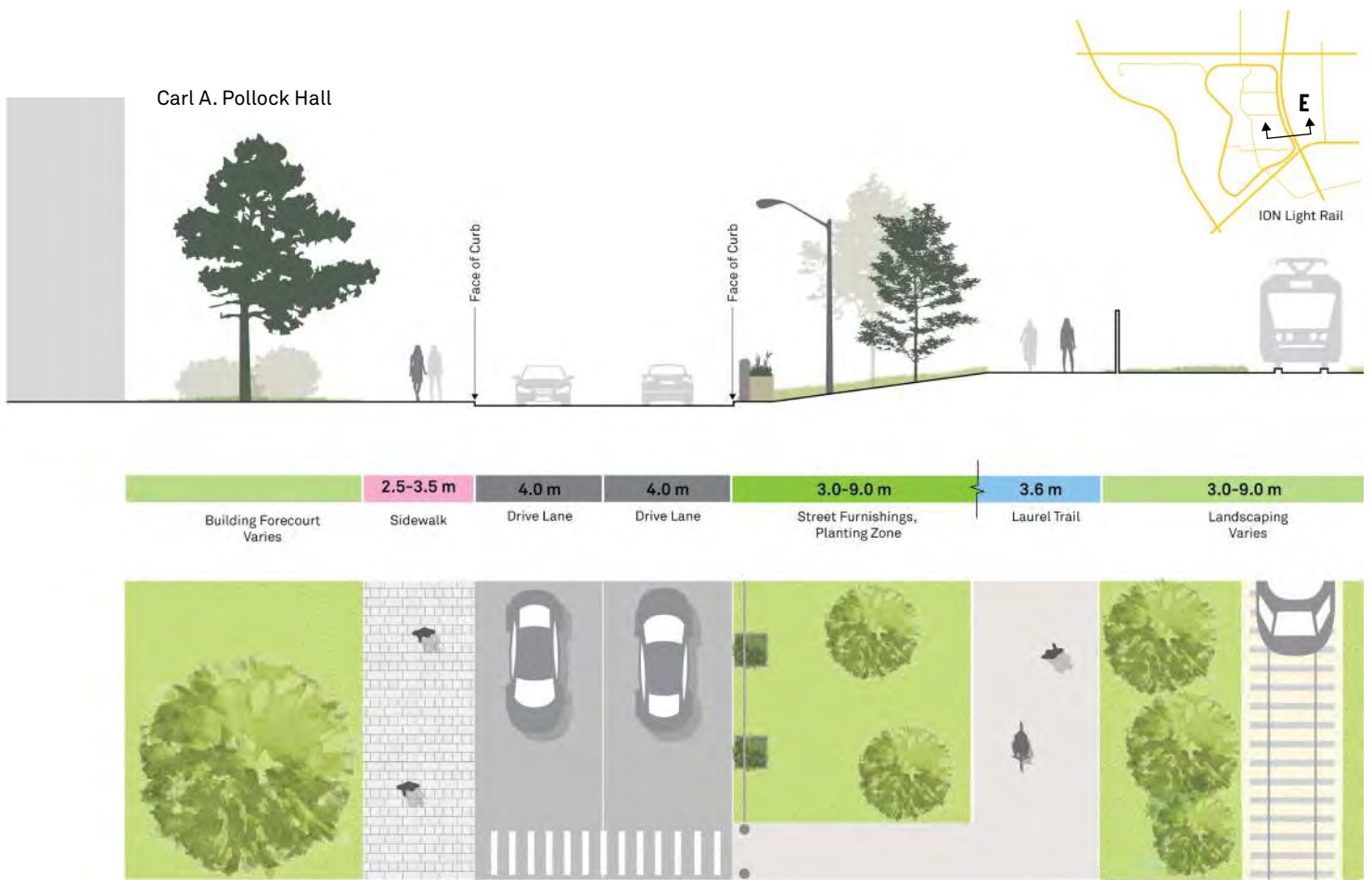
Figure 63. Section E. Existing condition of Ring Road (southeast edge).
