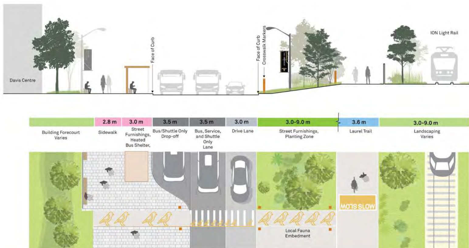
Figure 62. Section D. Proposed condition of Ring Road (eastern edge).
