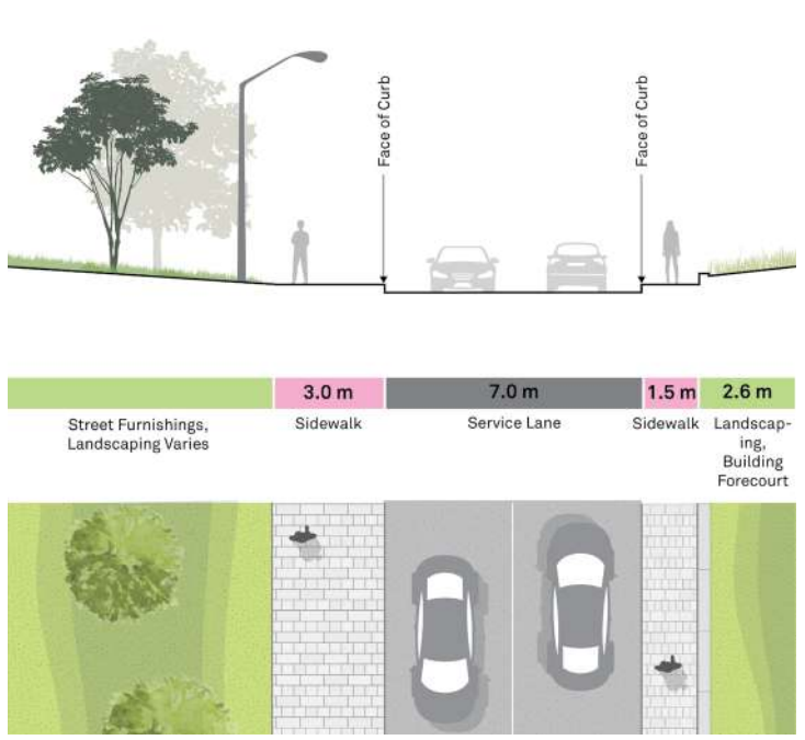
Figure 69. Section H. Existing condition of Engineering Service Lanes between DC and E3
