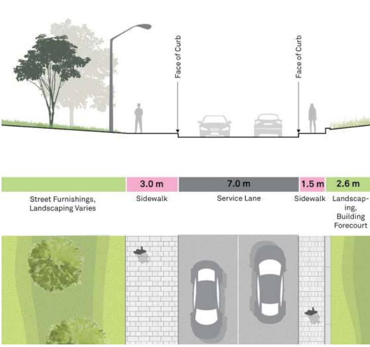
Figure 69. Section H. Existing condition of Engineering Service Lanes between DC and E3
