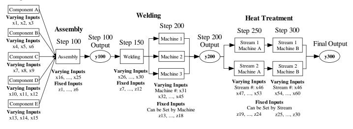
The Watfactory virtual process simulates a manufacturing process for automobile camshafts and has a number of processing steps and many inputs – see process map above. The process has 60 inputs that vary in regular production (x1, ..., x60) and 30 inputs are normally fixed (z1, ..., z30). A web interface allows a wide variety of process investigations including many types of observational and experimental plans.
