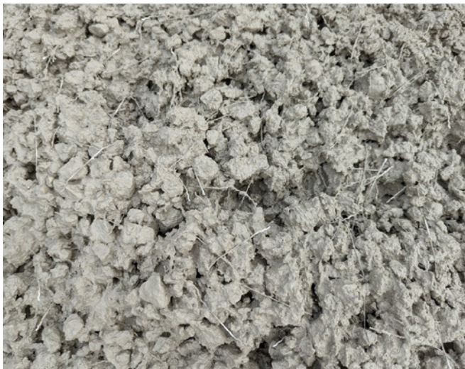
Above left: Fibre reinforced concrete closeup. Above right: Pouring concrete topping
