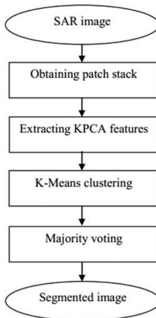
Figure 5. The flowchart of the proposed segmentation scheme.
