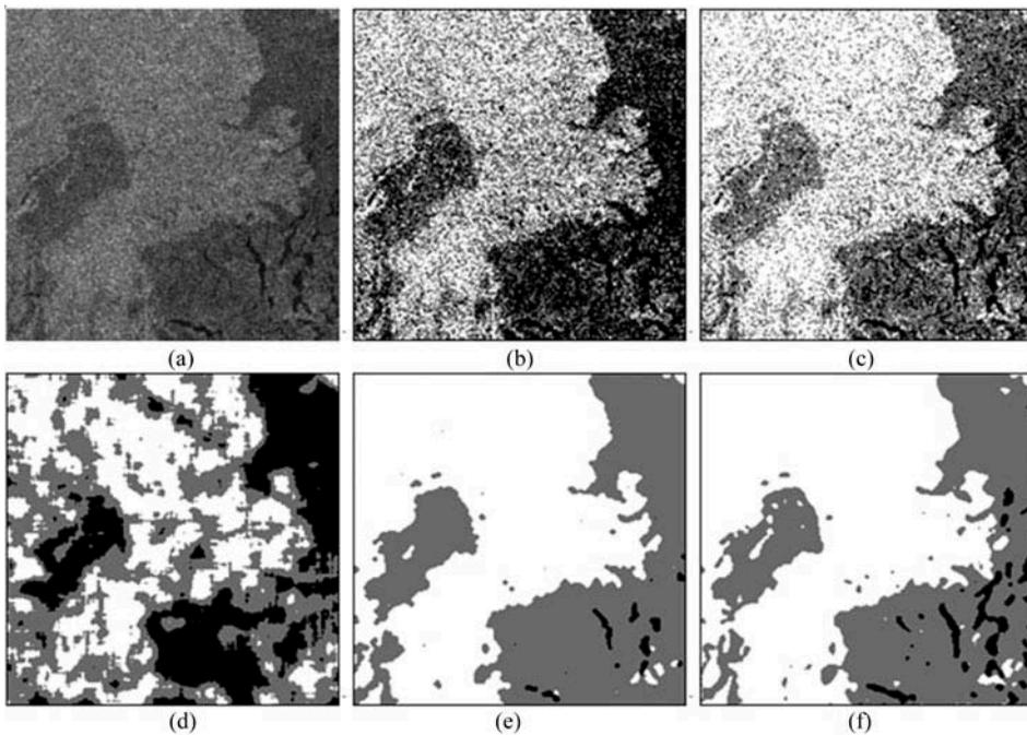
Figure 11. RADARSAT-2 images with three sea ice types labelled using each of the segmentation techniques. (a) Original image and images labelled using (b)  $k$ -means (c) log  $k$ -means, (d) GLCM, (e) MRF, and (f) KPCA techniques.
