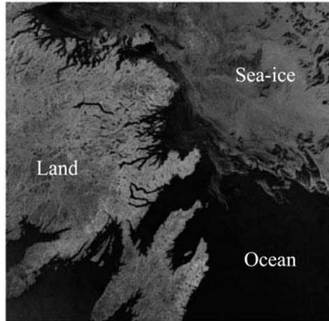
Figure 2. RADARSAT-2 image (7291 pixels  $\times$  7296 pixels) covering the sea area nearby the Island of Newfoundland in Canada, ScanSAR Wide beam mode, HH polarization, taken at 22:29:36 on 16 March 2009.
