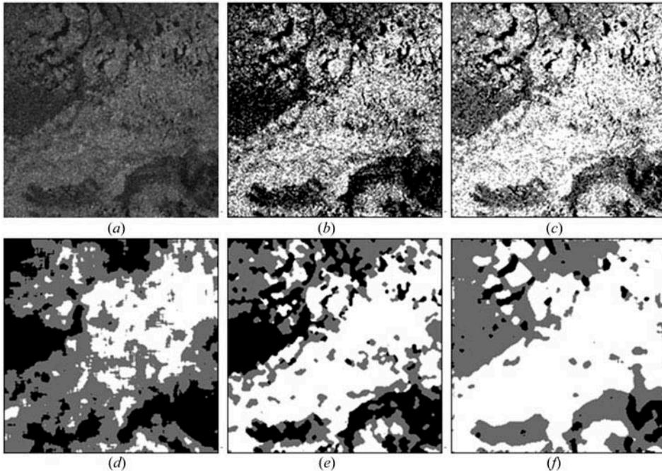
Figure 12. RADARSAT-2 images with three sea ice types labelled using each of the segmentation techniques. (a) Original image and images labelled using (b)  $k$ -means (c) log  $k$ -means and (d) GLCM, (e) MRF, and (f) KPCA techniques.
