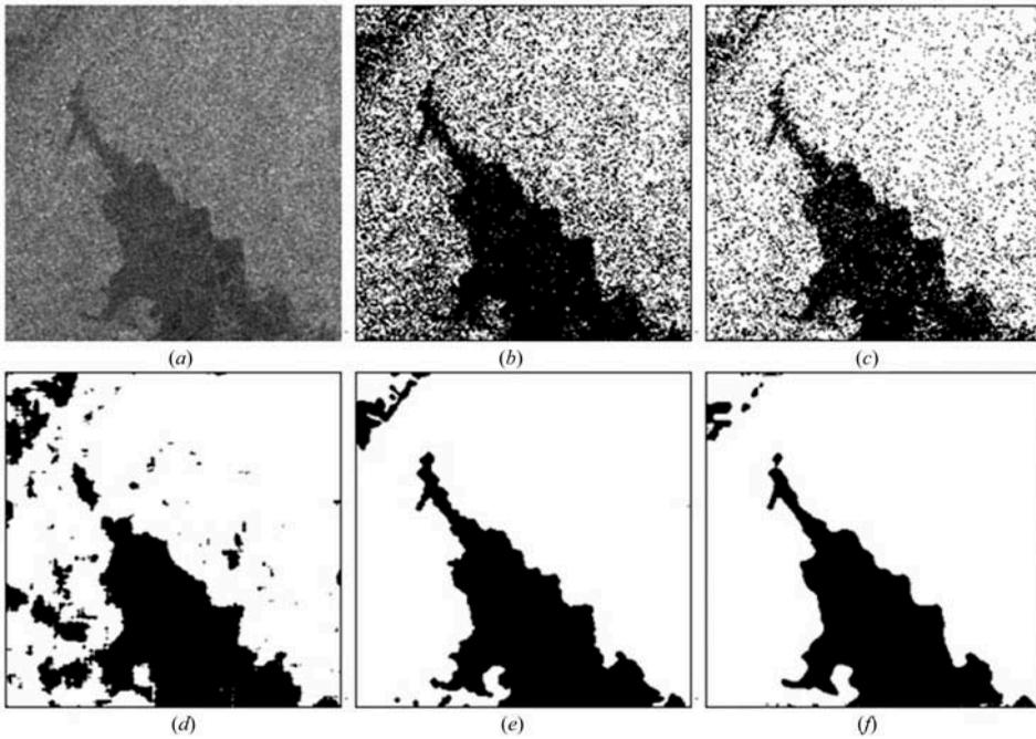
Figure 10. RADARSAT-2 images with two sea ice types labelled using each of the segmentation techniques. (a) Original image and images labelled using (b)  $k$ -means (c) log  $k$ -means, (d) GLCM, (e) MRF, and (f) KPCA techniques.
