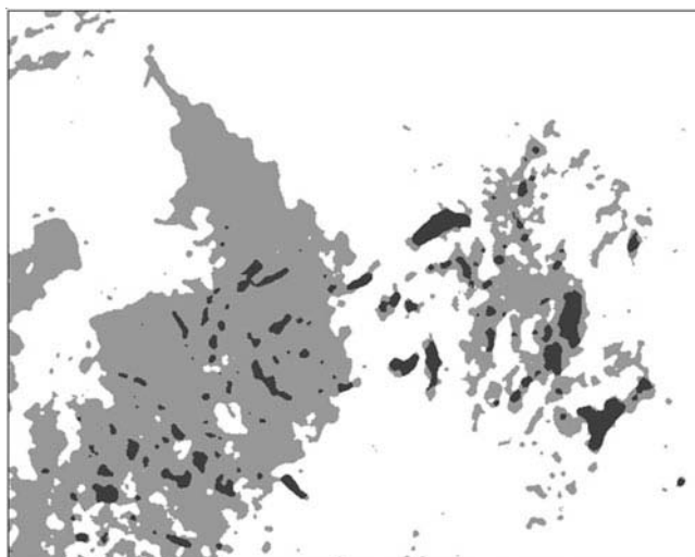
Figure 8. RADARSAT-2 images (684 pixels \times 544 pixels) with three sea ice types segmented using the proposed KPCA algorithm. Under the MATLAB platform, it took 1.77 s to process this image on a PC with an Intel ® 2.40 GHZ Quad-Core processor.
