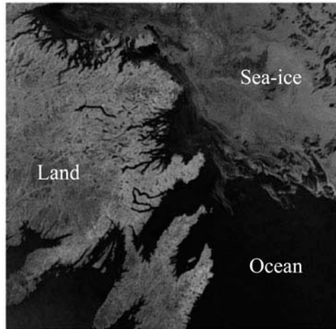
Figure 2. RADARSAT-2 image (7291 pixels \times 7296 pixels) covering the sea area nearby the Island of Newfoundland in Canada, ScanSAR Wide beam mode, HH polarization, taken at 22:29:36 on 16 March 2009.
