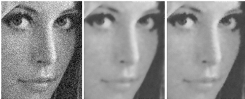
Fig. 3. TEST2: Left: Noisy image ( \sigma = 0.005 ), Middle: Isotropic NLM algorithm, Right: Proposed algorithm
