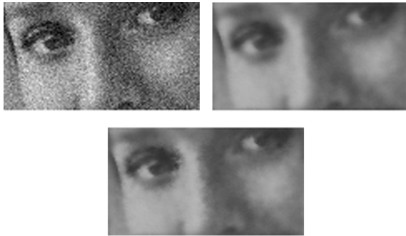
Fig. 4. TEST4: Top: Noisy image ( \sigma = 0.005 ), Middle: Isotropic NLM algorithm, Bottom: Proposed algorithm
