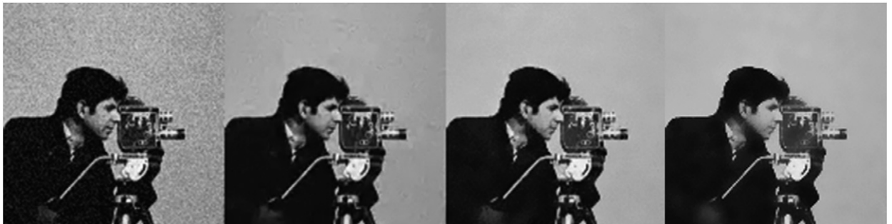
Fig. 1. CAMERAMAN test (from left to right): (a) noisy image, (b) Portilla method, (c) proposed method, and (d) bilateral filtering.
