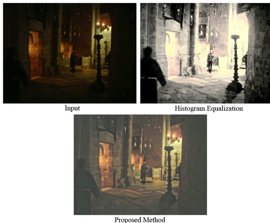
Figure 5. Color image enhancement results for Color Test 1 [11] for the proposed method and histogram equalization. While both methods noticeably improves image contrast, the proposed method does a significantly better job at preserving the original photographic tone of the image. Furthermore, the image produced by the proposed method does not exhibit the strong blocking artifacts visible in the image proposed by color image histogram equalization.
