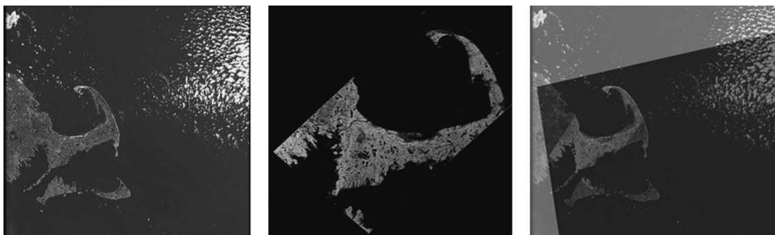
Fig. 7. Image registration from INTER5 test set. (Left) Reference image. (Center) Sensed image. (Right) Aligned images.
