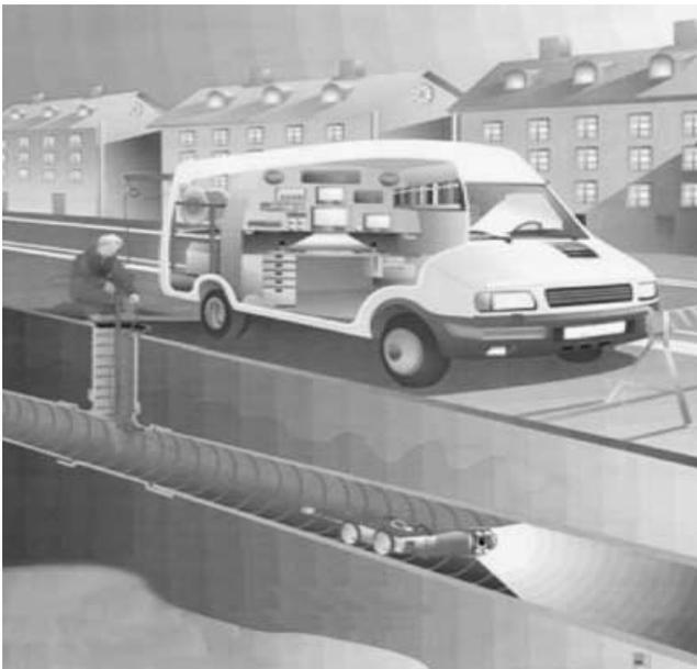
**Fig. 5.** CCTV camera inspection process of underground concrete pipe.
