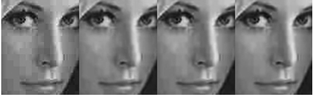
Figure 4. Part of JPEG-compressed “Lena” image (from left to right): a) decompressed image, b) deblocked using the Nosratinia method [13, 15], c) deblocked using the Wong method [16], and d) deblocked using the proposed method.
