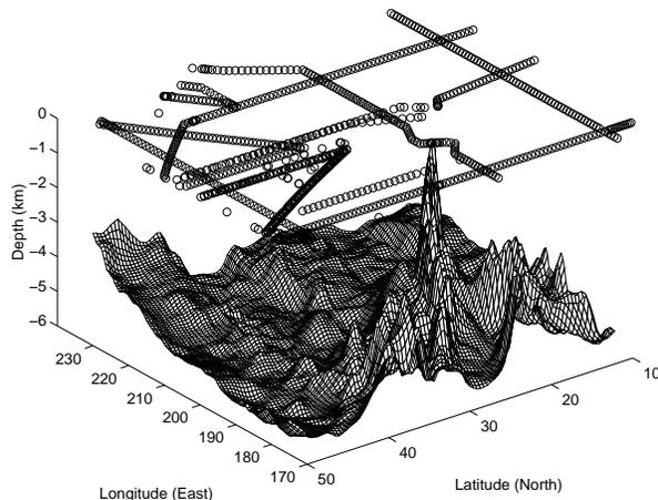
Figure 1: The Pacific basin bathymetry and sparse measurement distribution (measurements are taken at all depths below each circle).
