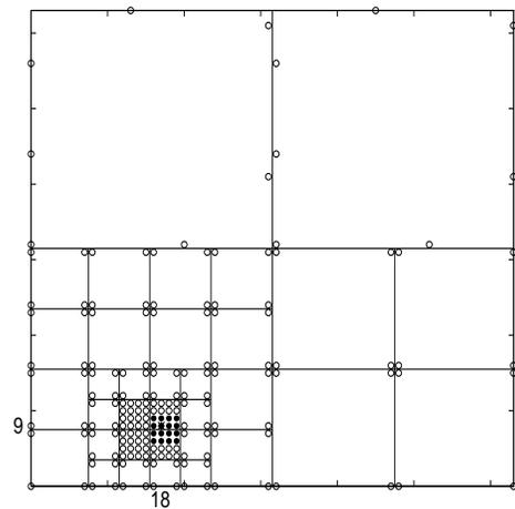
Figure 7: One possible limiting case of Figure 6 for estimating the single pixel (18,9). The state elements are either individual pixels (solid circles) or local averages of pixels (open circles).
