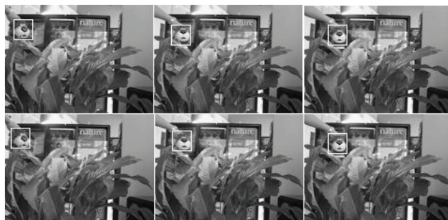
Figure 4: Result similar to Figure 3: Top row shows TCRF prediction in frames 3, 8 and 11. Bottom row shows template matching results. The object being tracked, the animal's face, is changing, since the face is turning. (This dataset was copied from www.vision.ucsd.edu/bbabenko )
