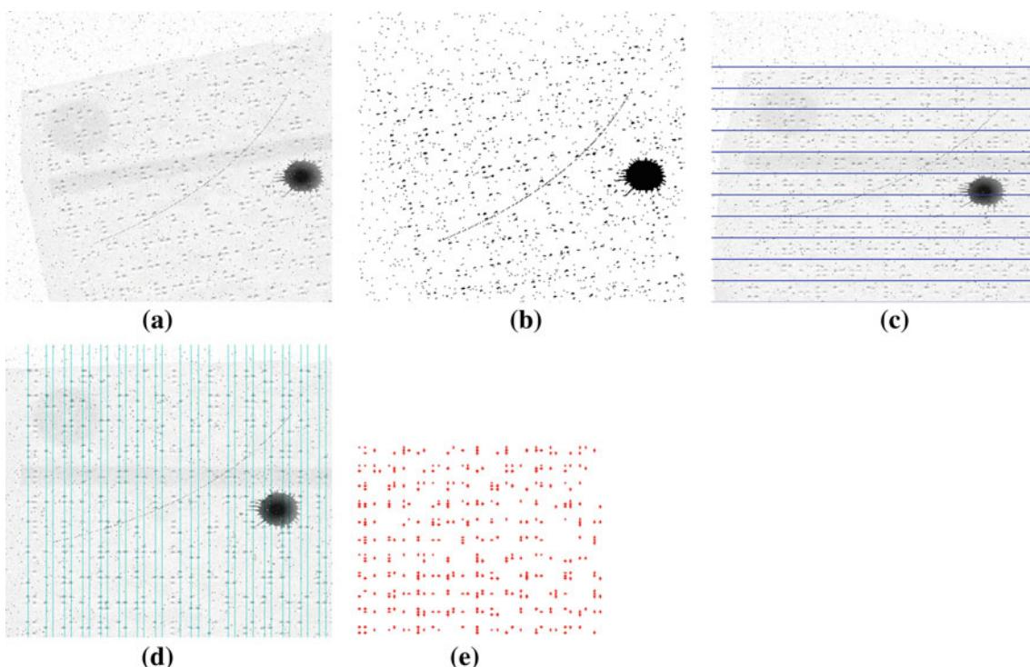
**Fig. 10** **a** A portion of a noisy Braille document with corresponding skewness of  $15^\circ$ , **b** the corresponding binary image, **c** the skewness is corrected and lines are separated, **d** the line parameters are detected, **e** the final estimation of Braille dots
