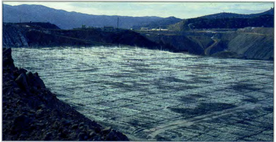
Acid leaching of copper ore, Ray Copper Mine, Arizona. All water on the mine property must remain there or be allowed to evaporate, with no runoff.
