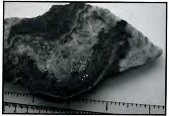
Figure 2: Electrum grains (lightest color) within acanthite (light color) layer in silver black band composed of chlorite, pyrite, chalcocopyrite, sphalerite and galena are 1 mm in diameter.
