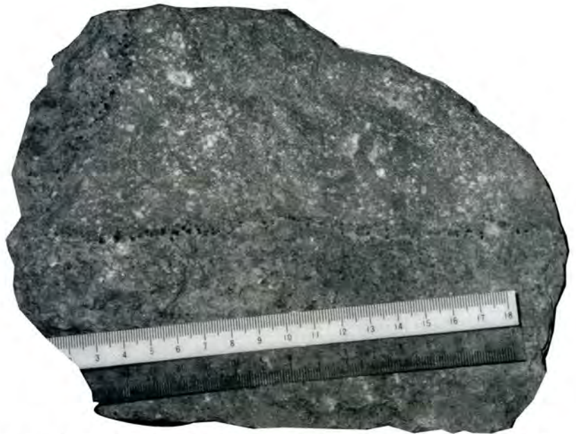
Figure 5: Gold ore from the Akeshi Mine. In the upper half of the sample, large vugs are filled with sulphur and the silicified rock is indicated by the light colour. In the lower half of sample, there is no sulphur and the rock is very porous. Covellite (a copper sulphide) or pyrite (iron sulphide) is concentrated at the boundary between two zones.
