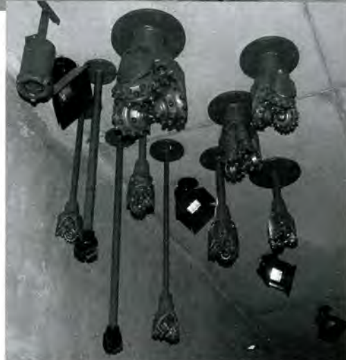
The drill-bit ceiling area: Poking through the ceiling are various diameter drill bits that are used for drilling, water, oil and gas wells. These bits were donated by Security DBS, Calgary, Christiensen Mining Products and Walker McDonald Bits. They are mounted to show how they would look from below as they make their way through rock strata deep underground.
