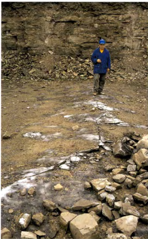
Figure 3. Peter is standing on the crestline of a pop-up in Dundas Quarry
