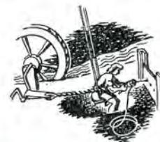
Drawing copper wire by water power in the 16th century.
