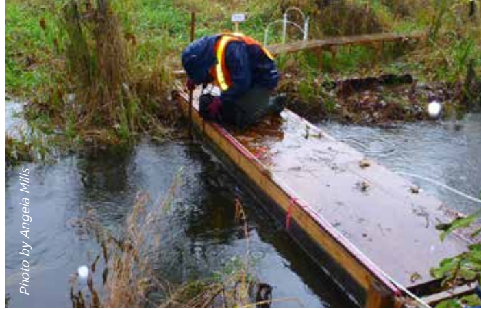
Collecting velocity and discharge measurements in the rain.
