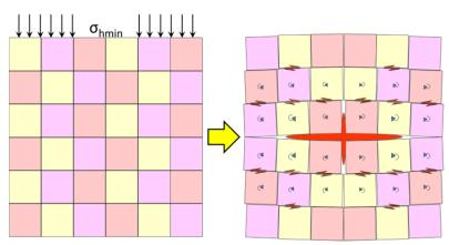
Forcing open a fracture near the injection point leads to rock block slip and joint opening far from the propped region (shown in red), and this effect, combined with the even more distant hydroshearing, leads to a stimulated zone that is much larger than the propped zone. Of course, the natural fractures are not so regular as in an array of child's blocks, but the processes of hydrofracturing and hydroshearing are the same. A more realistic figure of the stimulated zone is shown below.
