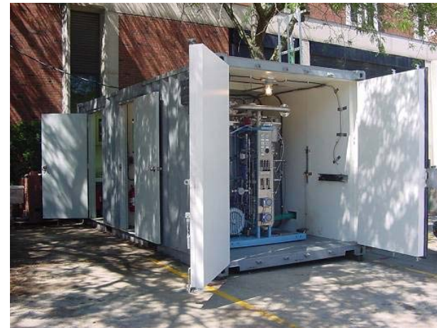
Pilot-Scale VaPRRS in Shipping Container
