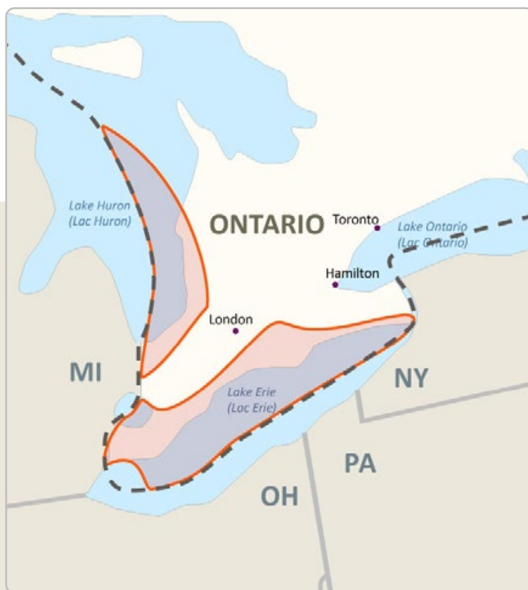
Figure 2: Map illustrating the suitable storage formations in southwestern Ontario for carbon storage.
