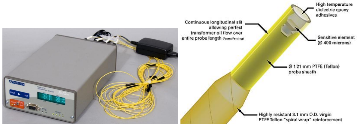
Figure 3-16: Optic thermal sensors (in yellow) connected to the measurement unit.
