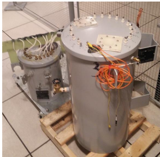
Figure 3-3: A photograph of model transformers, (left): original transformer, T1 (right): scaled transformer, T3.
