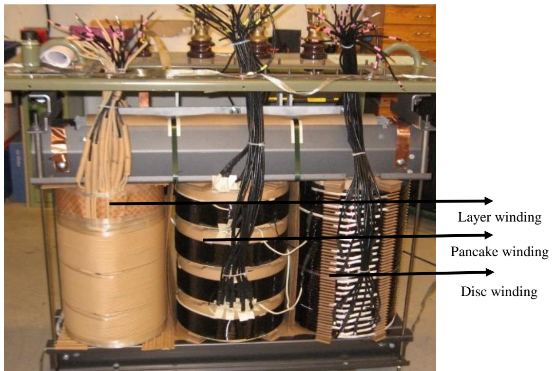
Figure 3-6: T5 model transformer (un-tanked), showing different winding types and connection leads.
