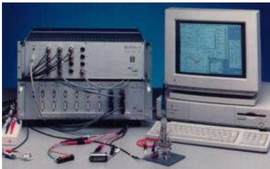
Bio-Logic Science Instrument: MacPile II Galvanostatic/Potentiostatic Multichannel Analyzer
