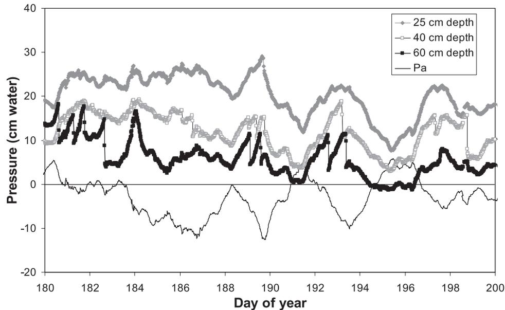
**Figure 5.** Variation of excess pressure  $P_e$  in three levels at site C and deviation of atmospheric pressure  $P_a$  from 101.3 kPa (= 1033 cm water) in 2003.
