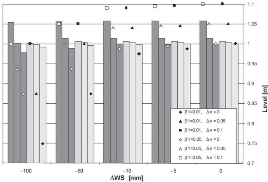
**Figure 6.** Calculated levels of water table and surface in a 1 m thick peat profile under conditions with different volumetric gas content ( $\Delta\gamma$ ), peat compressibility ( $\beta_1$ ), and size of water storage change ( $\Delta WS$ ) from a totally saturated soil. Bars represent surface level (dark for  $\beta_1 = 0.05 \text{ kPa}^{-1}$  and light for  $\beta_1 = 0.01 \text{ kPa}^{-1}$ ), while symbols represent water table level.
