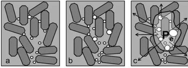
**Figure 1.** Conceptual model of bubble entrapment. (a) Bubbles get stuck in cavities and to pore walls by adhesion forces. (b) There they accumulate and grow, in such an extent that (c) they may restrict the movement of both water and gas and closed zones or layers may develop. Such confining layers may further trap locally produced peat gas, creating overpressured zones within the peat ( $P_e$ ).
