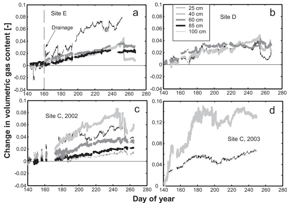
**Figure 3.** Change in volumetric gas content since the seasonal start of measurements at (a) site E, (b) site D, and site C (c) in year 2002 and (d) in year 2003. Dashed line in Figure 3a denotes the day of drainage (day 161).
