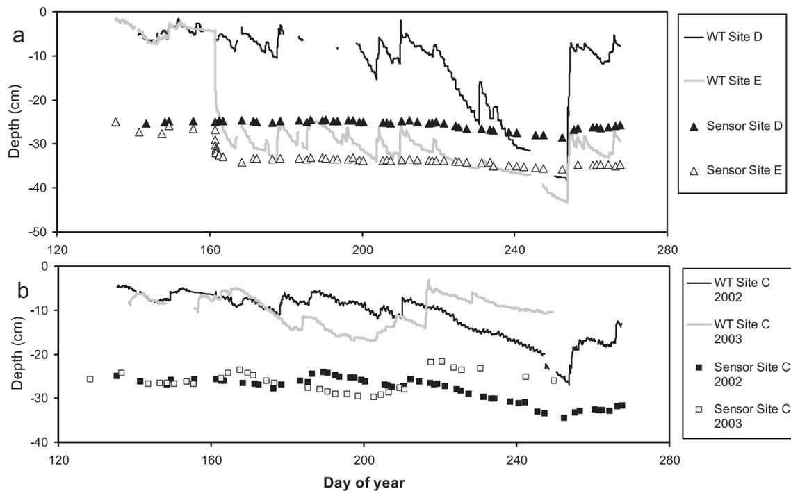
**Figure 2.** Variation of water tables and levels of moisture sensors installed at 25 cm depth (a) at sites D and E and (b) at site C.
