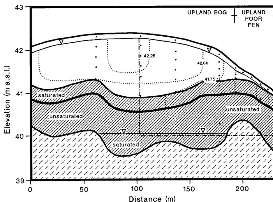
Figure 5. Observed 'steady-state' flow regime for upland blanket peat complex. See Figure 1 for material legend. Observed equipotential lines are given as dotted lines: ● = permanently installed piezometers; ▲ = permanently installed wells
