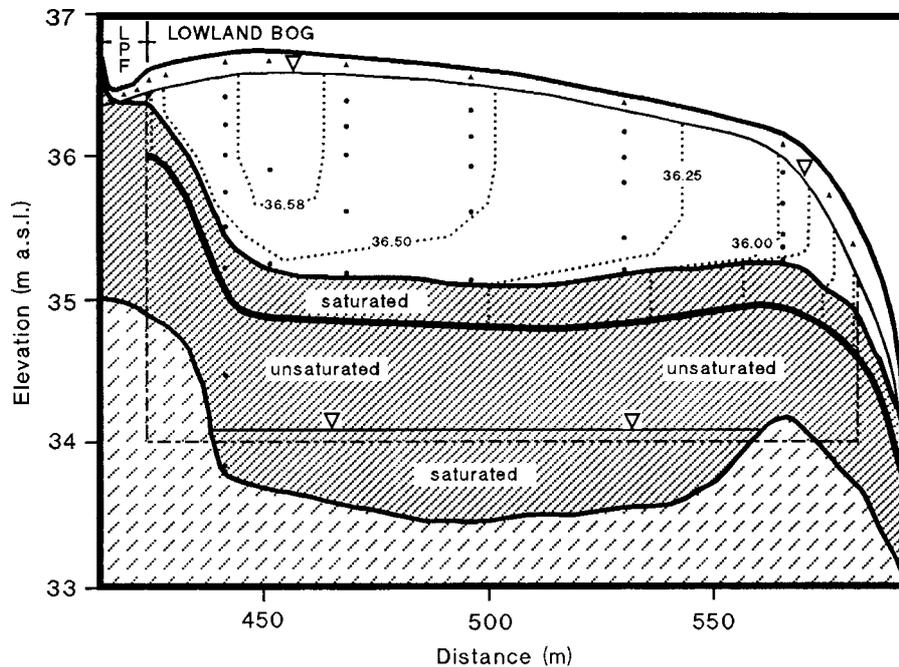
Figure 4. Modelled 'steady-state' flow regime for lowland blanket peat complex. Modelled flow regime was superimposed on Figure 3 site map. See Figure 1 for material legend. Equipotential lines are given as dotted lines ● = permanently installed piezometers, ▲ = permanently installed wells
