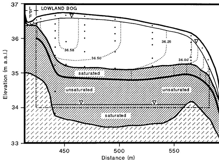
Figure 3. Observed 'steady-state' flow regime for lowland blanket peat complex. See Figure 1 for material legend. Equipotential lines are given as dotted lines: ● = permanently installed piezometers; ▲ = permanently installed wells
