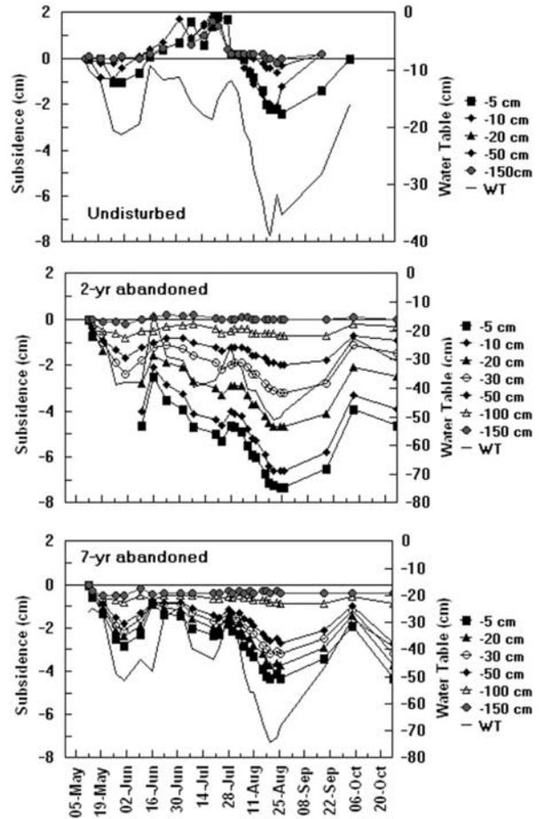
**Figure 4.** Sensor displacement plotted relative to initial position on 15 May for (top) undisturbed, (middle) 2-year, and (bottom) 7-year abandoned sites. Water table at each site is also shown. See color version of this figure in the HTML.
