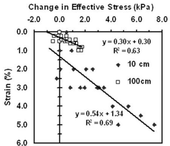
**Figure 7.** Changes in effective stress versus strain in the 5–10 cm layer and 100–150 cm layer in the 7-year abandoned site. Stress was determined from equation 1, and strain was derived from the soil deformation sensors. The poor resolution (0.5%) of the strain measurements is reflected in the horizontal distribution of points (range of  $\sigma_c$  for a given strain) in Figure 7.
