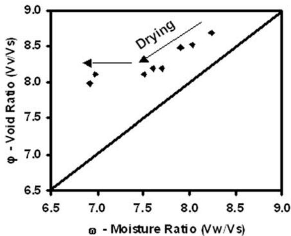
**Figure 8.** Laboratory results of volume change in a drying peat sample. The solid line represents normal consolidation in a completely saturated medium. The data are parallel to this line, indicating normal consolidation but incomplete saturation.
