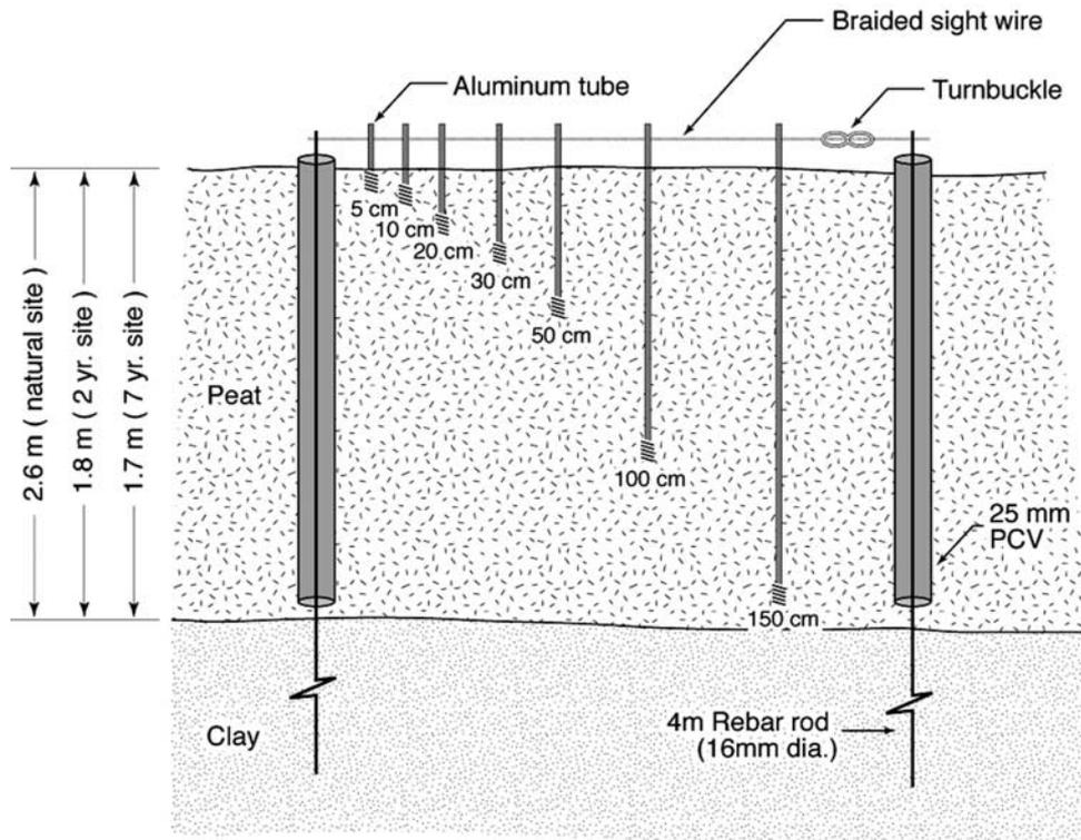
Figure 1. Soil deformation sensor setup.
