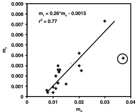
Figure 3. Virgin compressibility versus recompression ( $\text{kPa}^{-1}$ ). Regression was calculated ignoring the encircled point. Including the encircled point, the regression was  $m_r = 0.17m_v - 0.0003$  ( $r^2 = 0.58$ )
