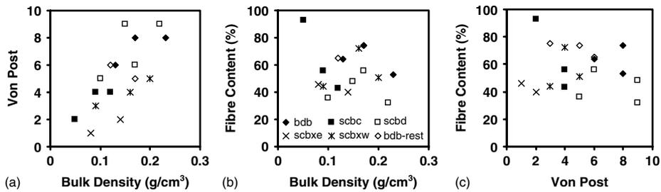
Figure 1. Bulk density versus (a) vP and (b) fibre content; (c) vP versus fibre content for peat from various sites
