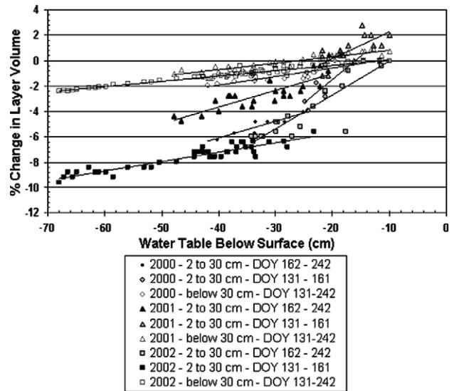
**Figure 2** Restored site wt below surface vs. % change in layer volume in zones of 5–30 cm and 30 cm and below for the 2000, 2001, and 2002 summer periods.
