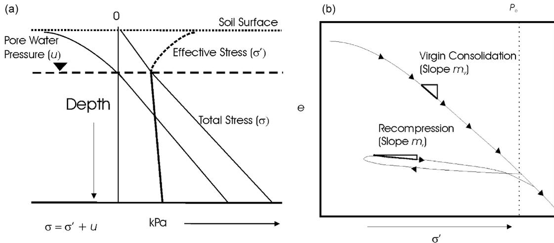
Fig. 1. (a) Effective stress concept, and (b) theoretical consolidation plot.
