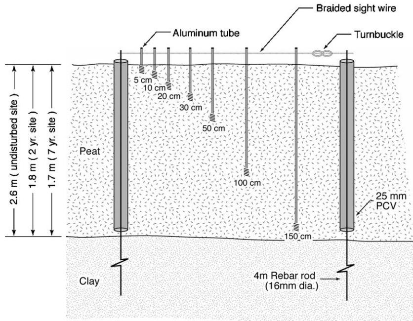
Fig. 3. Diagram of the peat elevation change measurement apparatus.
