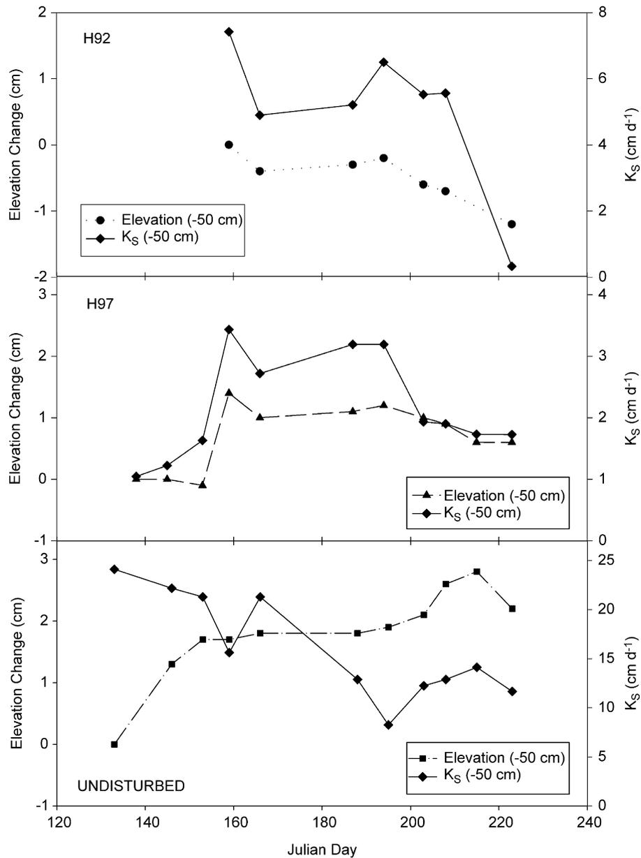
Fig. 7. Seasonal trends in elevation change and  $K_S$  at 50 cm depth at H92, H97, and UNDISTURBED.
