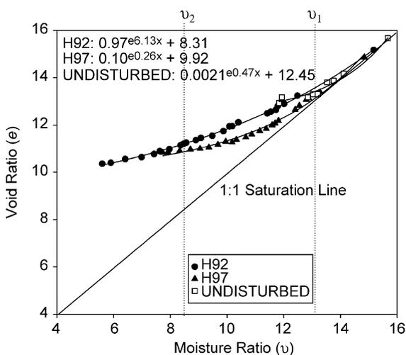
Fig. 6. The soil shrinkage characteristic at H92, H97, and UNDISTURBED sites.
