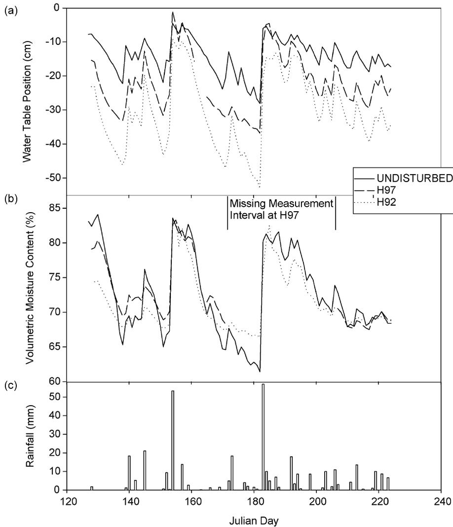
Fig. 4. (a) Water table, (b) volumetric moisture content at H92, H97, and UNDISTURBED sites and (c) daily precipitation.
