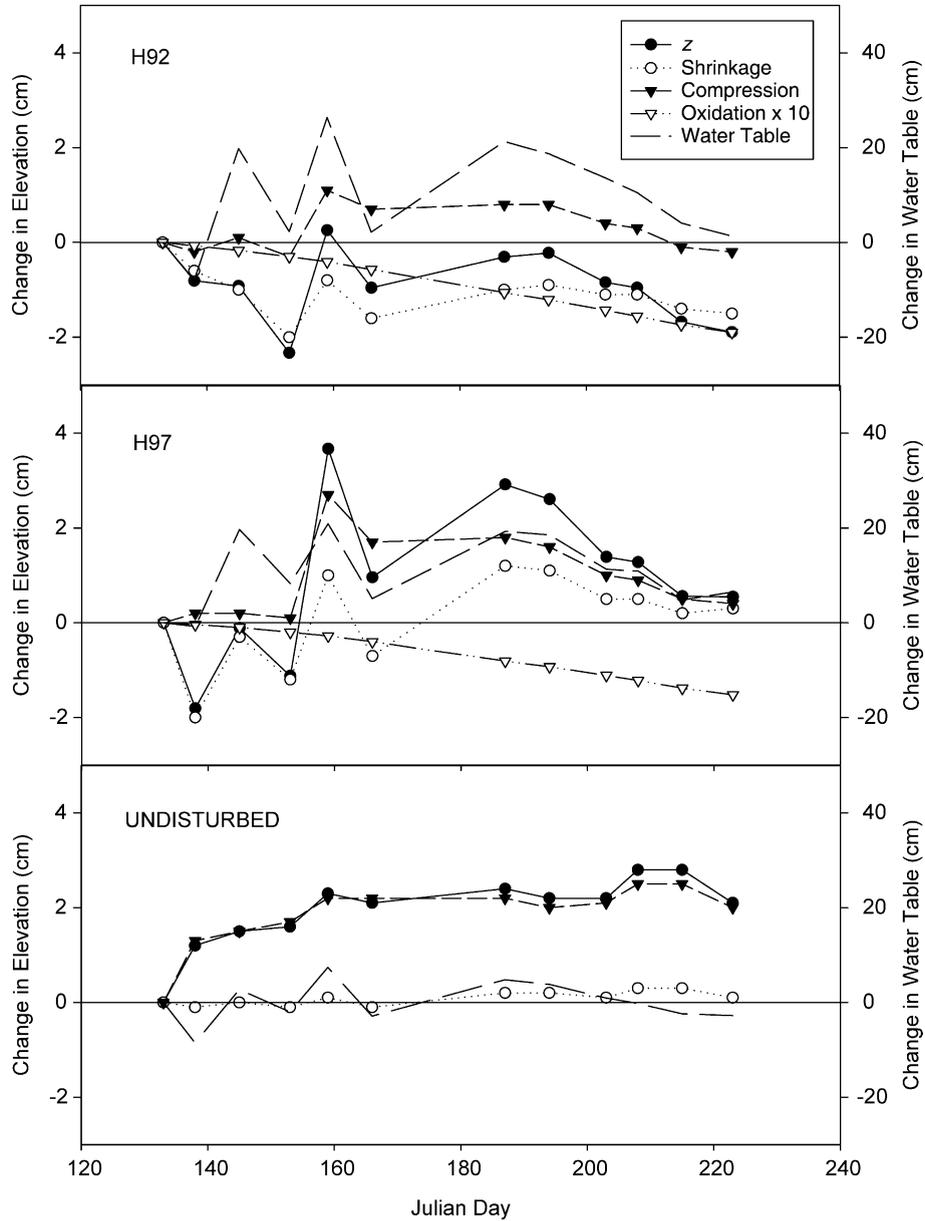
Fig. 5. Components of volume change at H92, H97, and UNDISTURBED sites.
