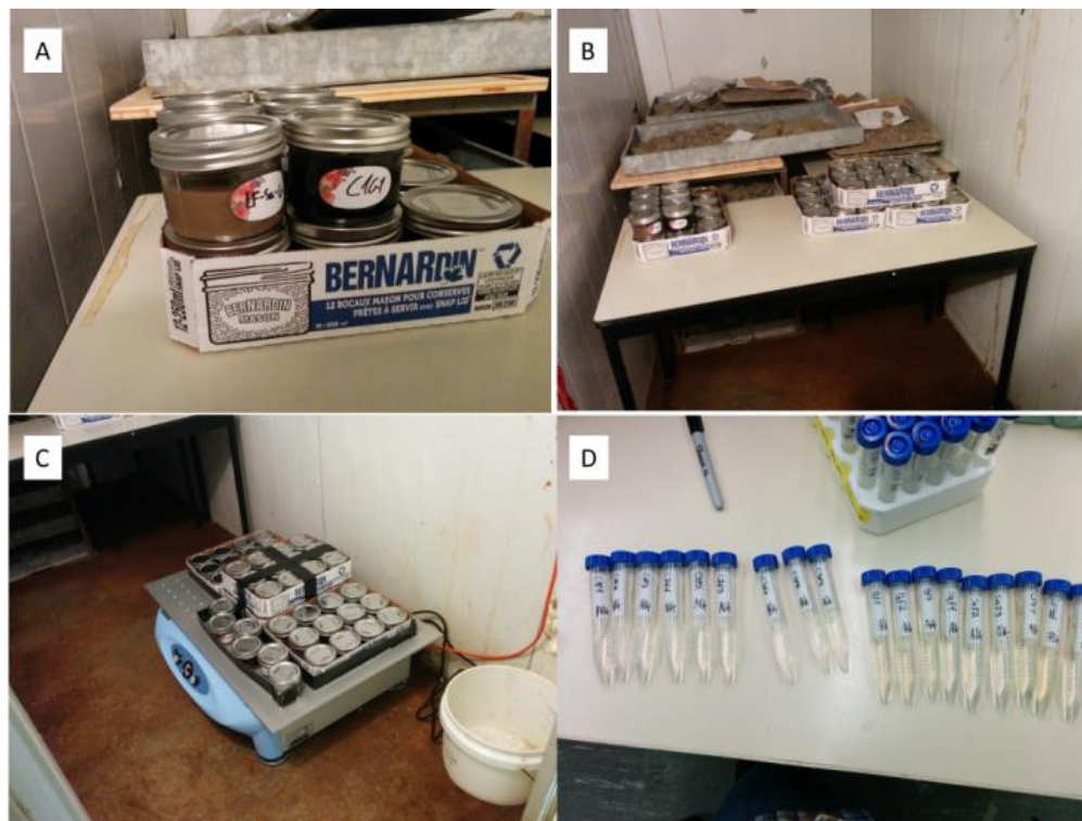
Figure A.1.3 - Pictures of incubation in the cold room from the leaching experiment. A) close up of incubation jars; B) all samples ; C) incubation jars on shaker; and D) samples after filtration and preservation for various analyses.
