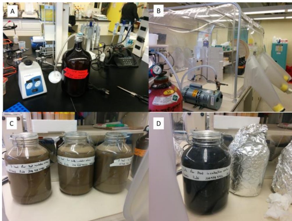
Figure A.1.2 - Pictures of solution preparation from the leaching experiment. A) Base solution purging with N_2 ; B) The anaerobic chamber used for preparations and sampling, base solution bottles can be seen in back of chamber; C) Jars with
